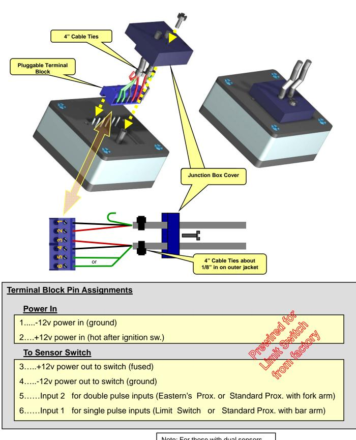
Note: For those with dual sensors Use input 1 & 2 where 1 is on before 2 in mixing direction
