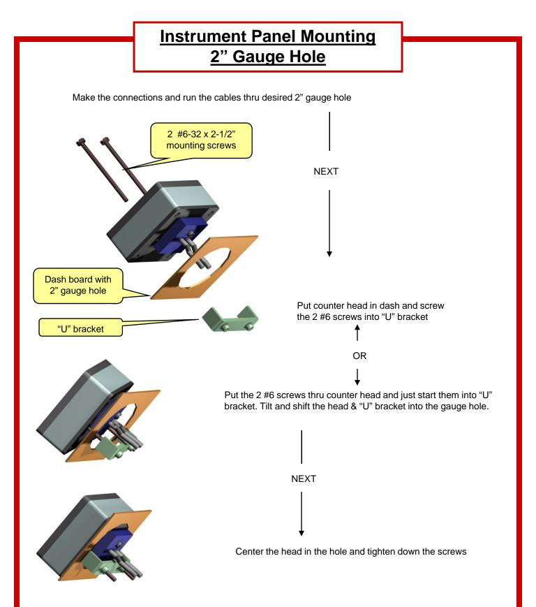
To remove the head in the future just remove 1 #6 screw completely and loosen the other. This will allow you room to tilt and shift the head & "U" bracket out.
